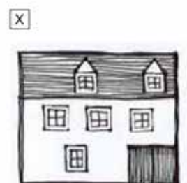
Loft conversion incorporating gabled dormers which are out of scale and do not consider existing window rhythm nor frequency.
